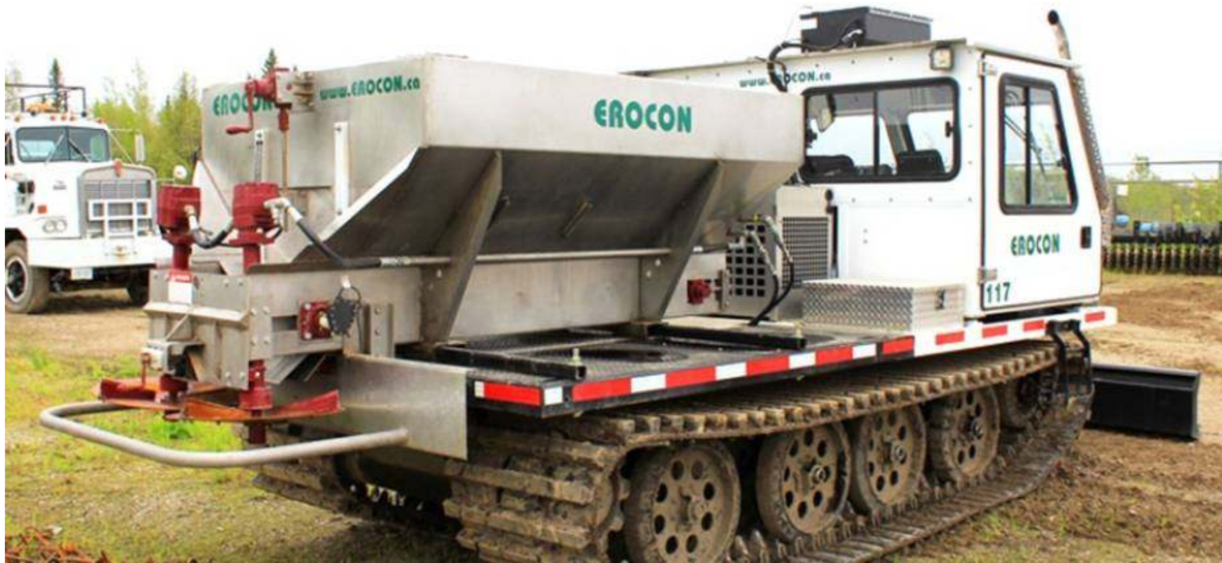
Lime Spreader / Hydro Seeder
