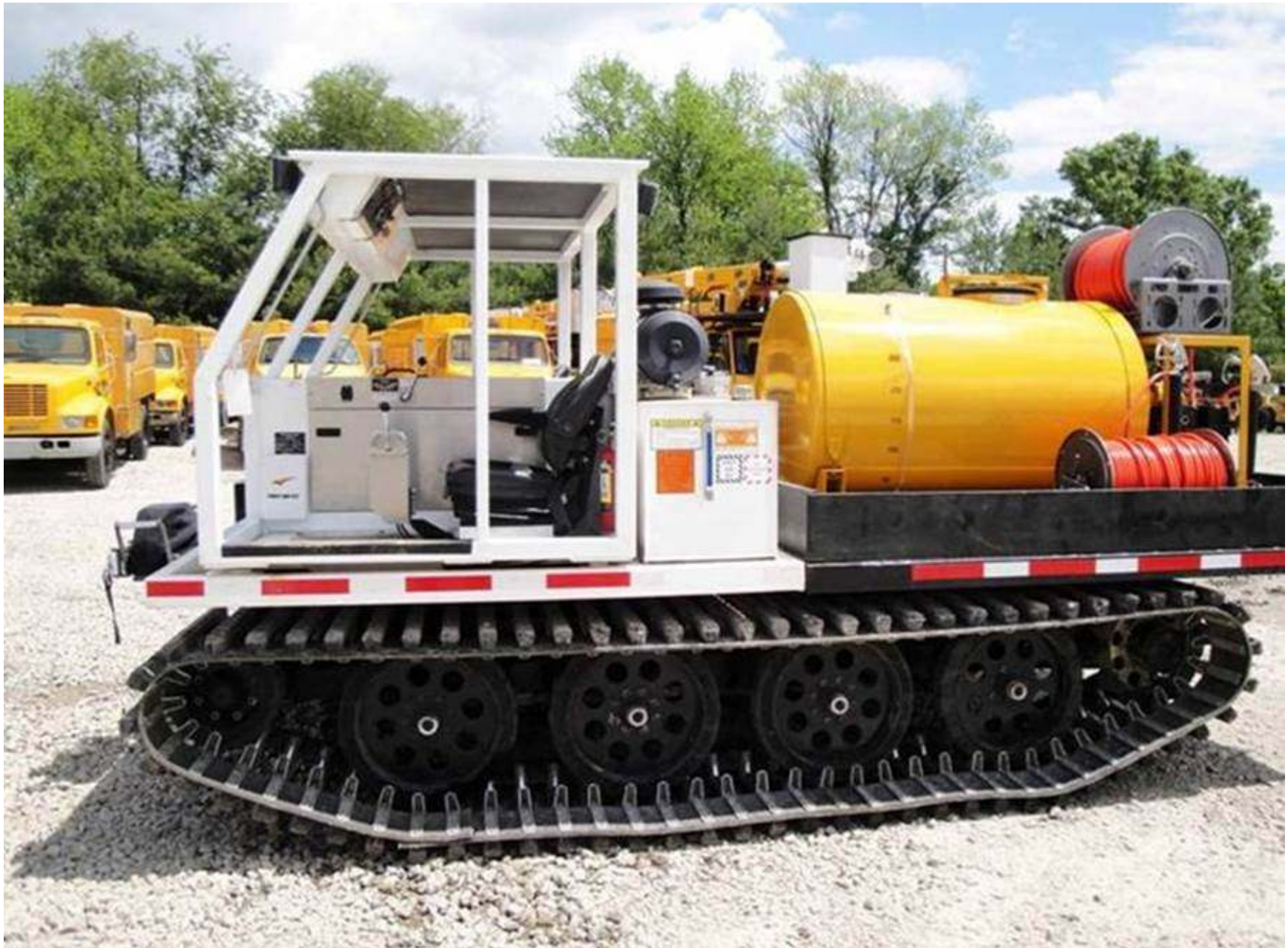
300 Gallon Spray Tank with Hose Reels - Customer Equipped
